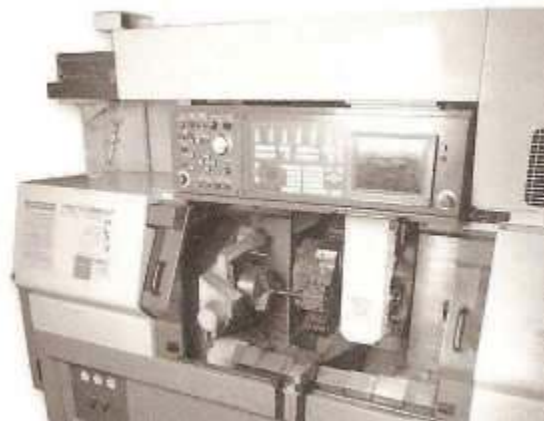
ISM's dual-turn lathe is capable of robotically loading and turning parts on each end simultaneously.
