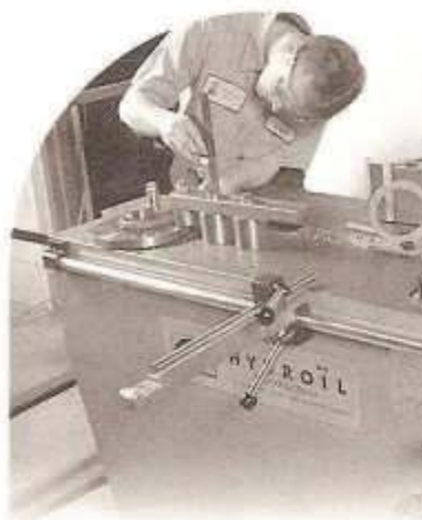
The business has the capability for rod, pipe and tube bending up to 2 inches in diameter.
